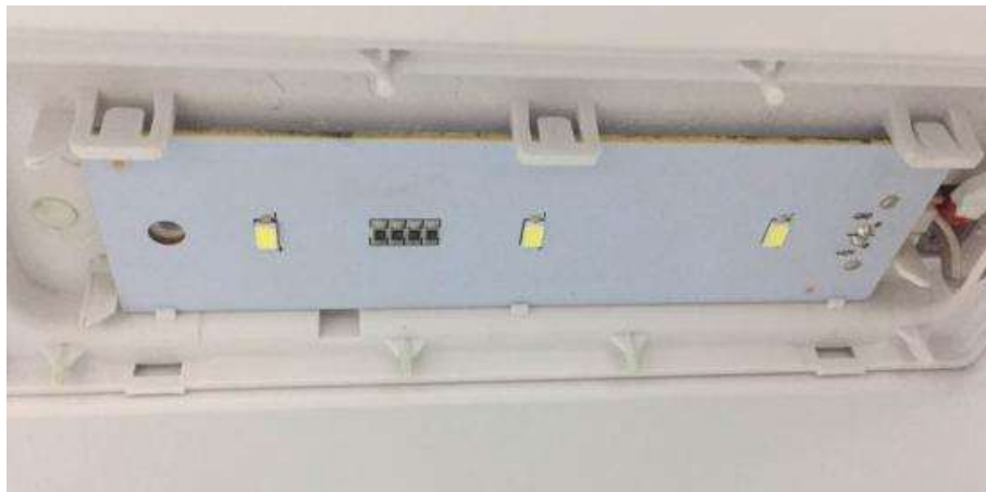
Front of LED PCB without cover (Model RD-40WC4SA2)
