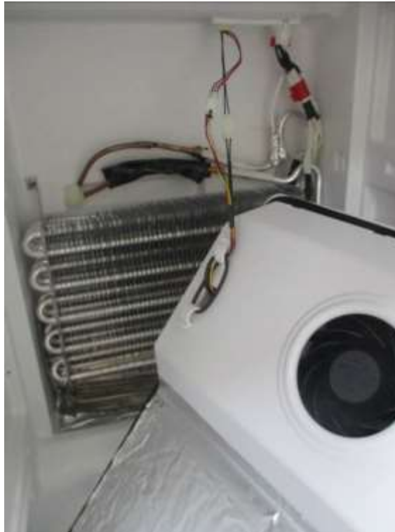
Freezer compartment internal view without cover
