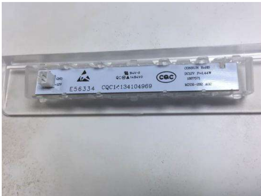
Back of LED PCB (Model RD-40WC4SB2)
