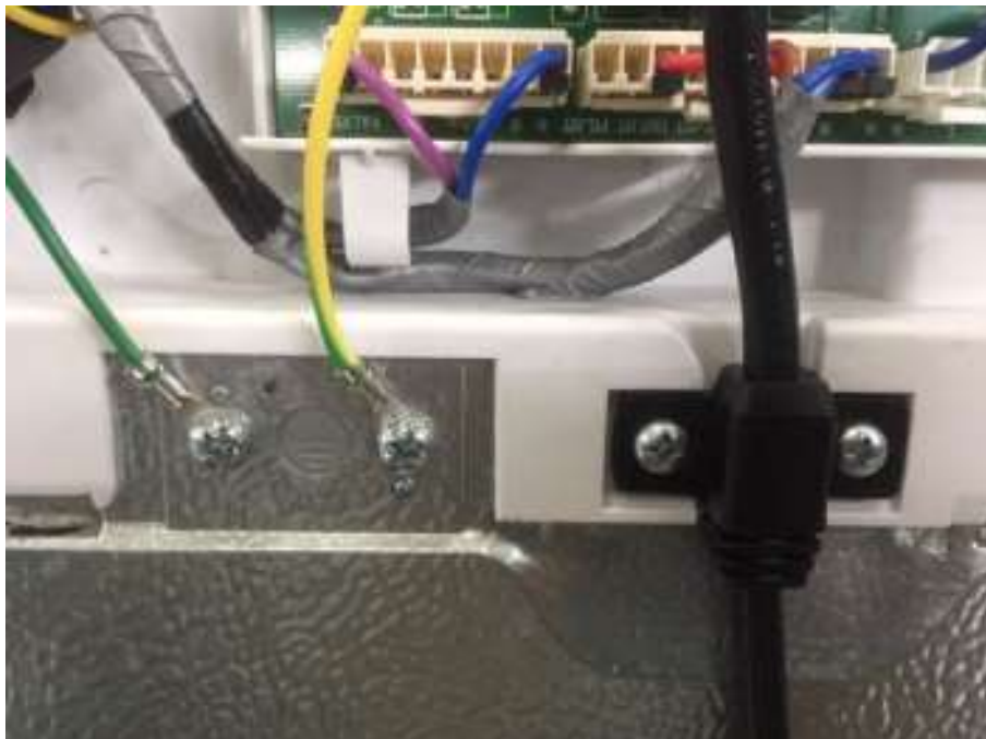
Earthing terminal &amp; Cord anchorage
