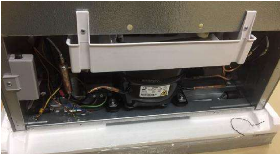
Compressor compartment (Model RD-40WC4SB2)
